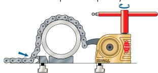
The chain length of 1 metre (longer on request) means you can clamp very large workpieces.
